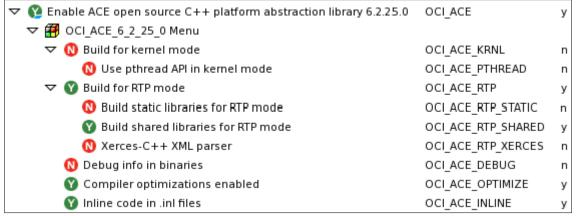
If Xerces-C++ was built (needed for DDS Security, see Building Xerces-C++ for VxWorks below), enable the OCI\_ACE\_RTP\_XERCES option and provide the path to the installed Xerces-C++ in the option below it. This is the directory above the "include," "lib," and "shared" directories created by the Xerces-C++ installation process. Use forward slashes on all host platforms.
